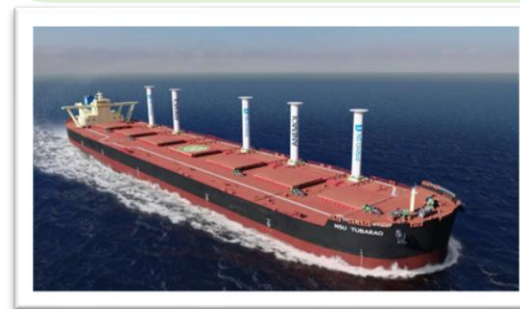
Image of Installed Rotor Sails on MV. NSU TUBARAO
