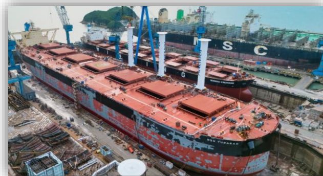
(Installed Rotor Sail)
