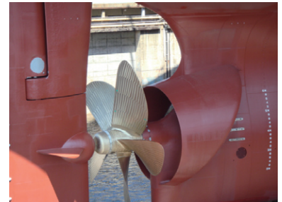
Energy-saving device mounted on the M/V SHIN-EI and M/V SHINWA-MARU Courtesy of Universal Shipbuilding Corporation
