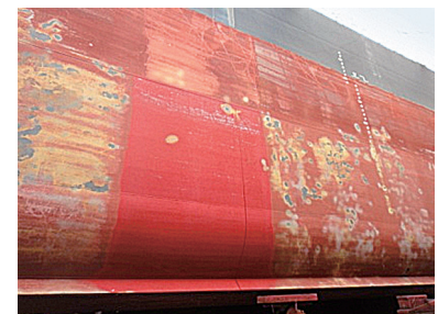
Fuel-efficient antifouling coating applied on M/V KIMITETSU-MARU
