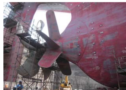
Energy-saving device mounted on the Yugawasan
