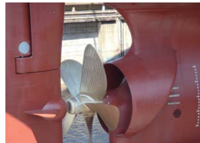
Energy-saving device mounted on the Shin-Ei and Shinwa-Maru Courtesy of Universal Shipbuilding Corporation
