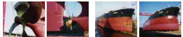
Before propeller polishing After propeller polishing Before hull cleaning After hull cleaning
