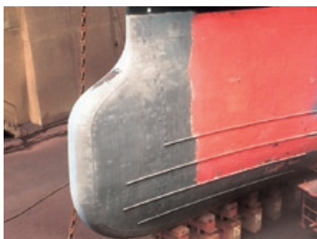
“FUYO MARU No. 5” in the process of paint stripping work on the bottom plating
