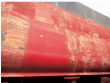
“KIMITETSU MARU” with fuel-efficient antifouling painting applied to the bottom
