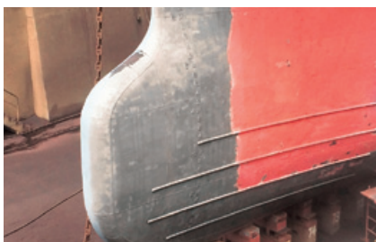
“FUYO MARU No. 5” in the process of paint stripping work on the bottom plating
