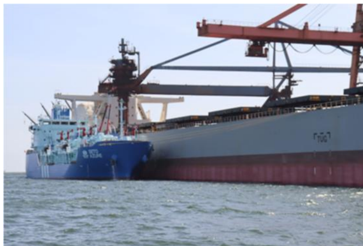
LNG bunkering using the STS Method by SETO AZURE (left)
